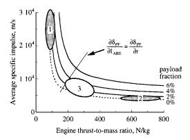
Fig. 1 Variation of payload fraction as a function of thrust-to-mass ratio and average specific impulse of engine: 1, airbreathing propulsion; 2, rocket propulsion; and 3, combined propulsion.
