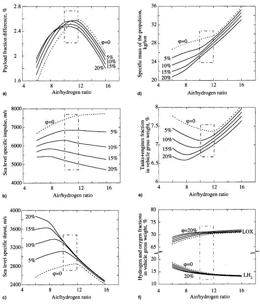
Fig. 9 Comparison of mass and efficiency parameters for LRE-DCTJ combined propulsion system with oxygen addition as a parameter.
