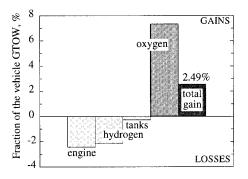
Fig. 10 Breakdown of payload fraction gain in KLIN cycle engine compared with a LRE vehicle.
