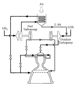
Fig. 2 Dual-mode LACE-M/LRE engine.
