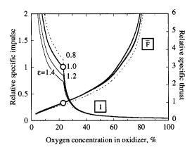
Fig. 6 Variation of relative specific impulse and relative thrust as a function of oxygen concentration in oxidizer with equivalence ratio as parameter.
