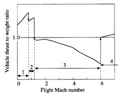
Fig. 11 Profile of the thrust-to-weight ratio for the lifting-body vehicle powered by KLIN cycle.
