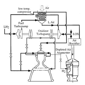
Fig. 3 LRE thermally integrated with air-separation system.
