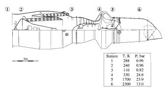
Fig. 8 Schematic of cryojet engine.
