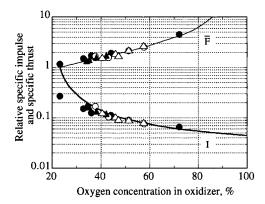
Fig. 7 Performance of different thermally integrated systems at equivalence ratio of unity. •, LACE-M, Ref. 5; ○, LRE + FLOX, Ref. 5; ▲, LRE + DCTJ, Ref. 6; and △, LRE + DCJ<sub>ox</sub>, Ref. 7.
