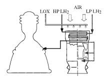
Fig. 4 LRE thermally integrated with DCTJ with oxygen addition, the KLIN cycle.
